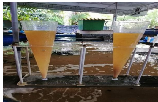
Figure 2: Measurement of biofloc concentration using Imhoff settling cones
