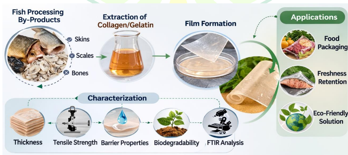
Fig. 2. Production and characterization of biodegradable packaging film from fish processing by-products
