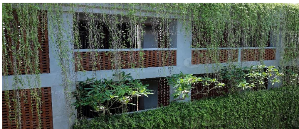
Figure: 4 Hanging-Down Green Wall
