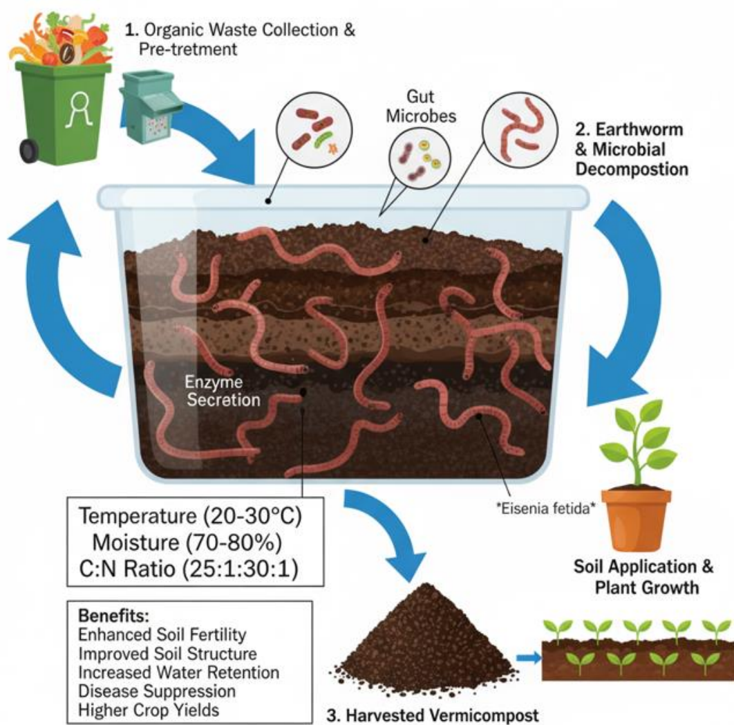
Figure 1. Schematic Diagram of the Vermicomposting Process
