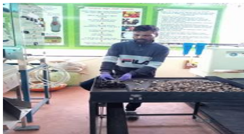
Fig 4: Hand cum pedal operated shell cutter
